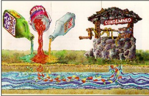
Contaminates discarded in a recharge area reaches the ground water aquifer and pollutes the well. Picture furnished courtesy of the Salt Lake County Water Conservancy District.
